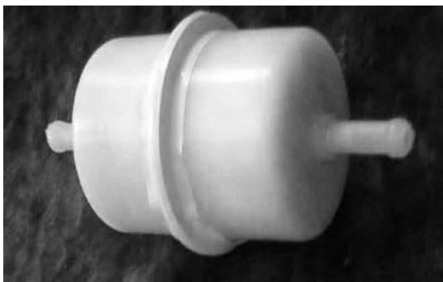
**Fig. 2.** Filtering cartridge with saline granules.
