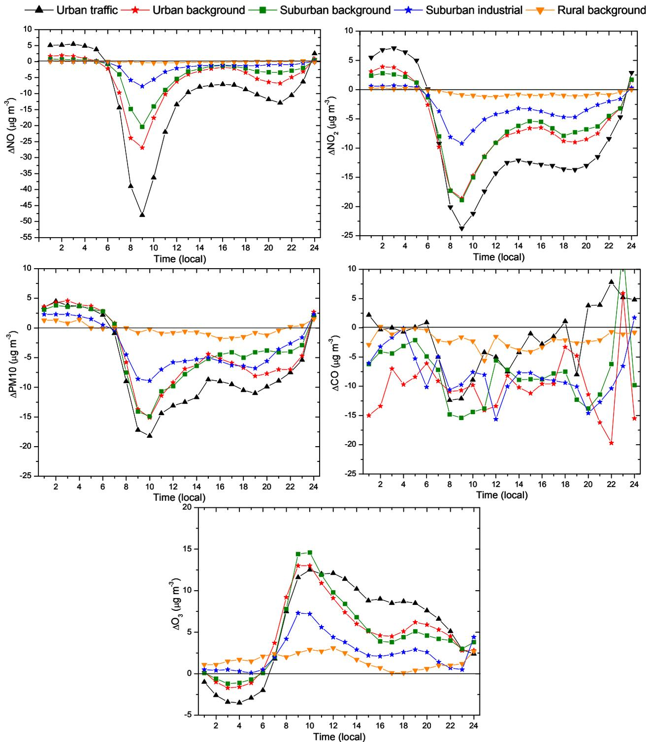
**Fig. 5.** Daily cycle of the differences (weekend minus work days) for O<sub>3</sub>, NO, NO<sub>2</sub>, PM<sub>10</sub> and CO as a function of the station type.
