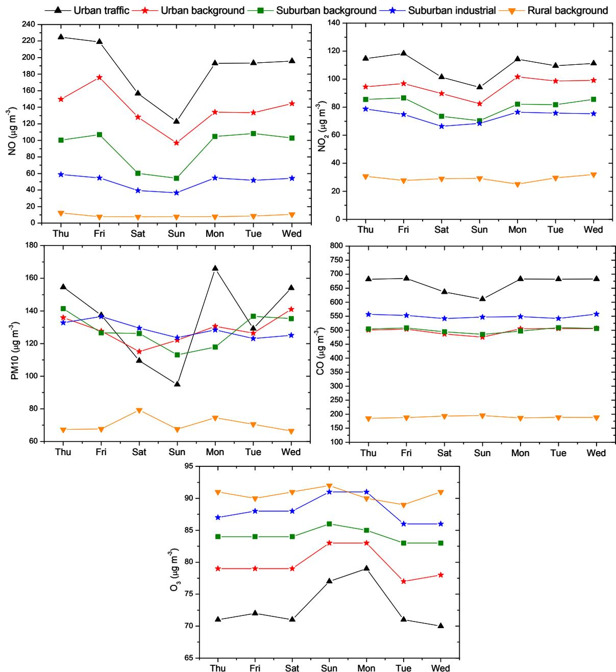
**Fig. 4.** Weekly patterns of maximum daily 8 hours mean for  $O_3$ , 90<sup>th</sup> percentile daily for  $NO$ ,  $NO_2$  and  $PM_{10}$ , and average daily for  $CO$  as a function of the station type.
