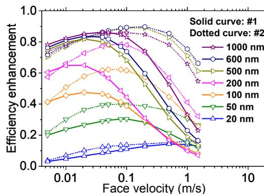
**Fig. 7.** Comparison of the variation of efficiency enhancement with increased face velocity for different particle sizes.
