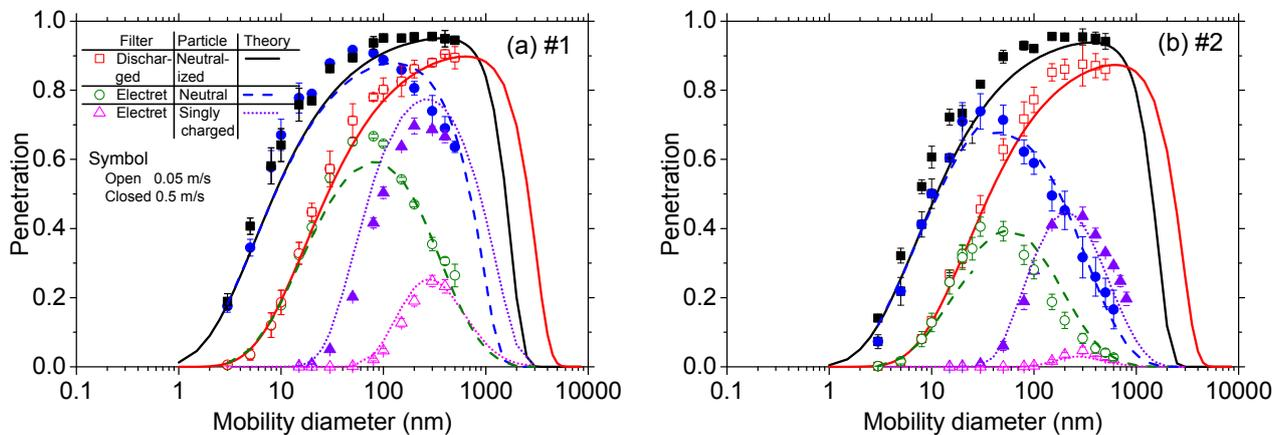
**Fig. 4.** Comparison of experimental and theoretical particle penetrations through Electret Filter #1 (a) and #2 (b) at face velocities of  $0.05 \text{ m s}^{-1}$  (open symbols) and  $0.5 \text{ m s}^{-1}$  (closed symbols). Squares represent the penetration of neutralized particles through discharged (mechanical) filter, circles represent the penetration of neutral particles through electret filter, and triangles represent the penetration of singly charged particles through electret filter.
