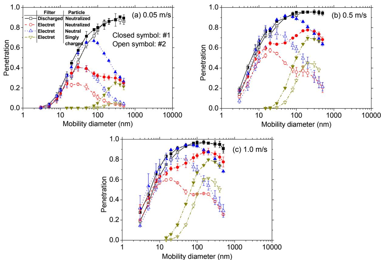
**Fig. 2.** The penetration of particles with different charge states through electret and discharged filter media at face velocities of (a)  $0.05 \text{ m s}^{-1}$ , (b)  $0.5 \text{ m s}^{-1}$ , and (c)  $1.0 \text{ m s}^{-1}$ .
