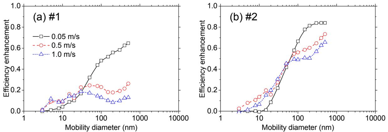
**Fig. 3.** Efficiency enhancement (differences in neutralized particle penetration) between Electret and Discharged Filter Media (a) #1 and (b) #2, due to the charge on fiber.
