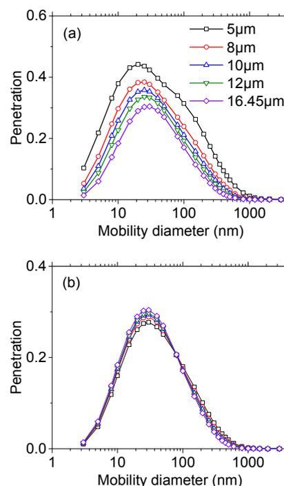
**Fig. 8.** Particle penetration as fiber diameter changes in electret filters kept at a constant pressure drop by (a) reducing fiber thickness and (b) reducing fiber solidity at face velocity of  $0.1 \text{ m s}^{-1}$ .
