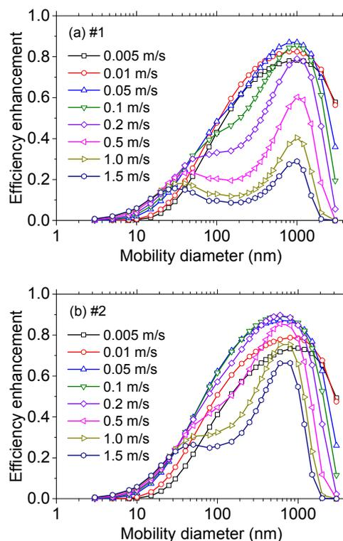
**Fig. 6.** Efficiency enhancement varied with face velocity in (a) Filter #1 and (b) Filter #2.
