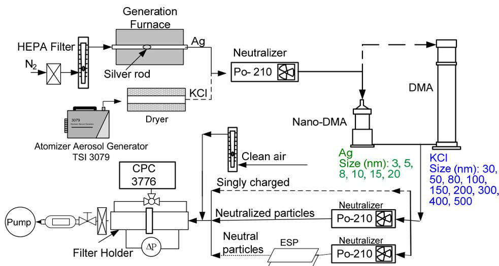
**Fig. 1.** Experimental setup for particle generation and filtration efficiency measurement.
