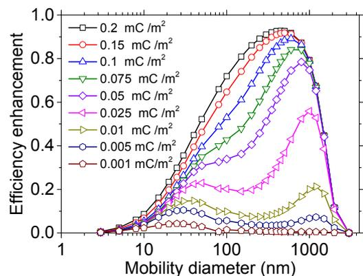
**Fig. 5.** Efficiency enhancement varied with fiber charge density at face velocity of  $0.5 \text{ m s}^{-1}$ .
