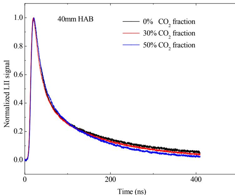
**Fig. 8.** Measured normalized LII signals at 40 mm HAB in different flames.
