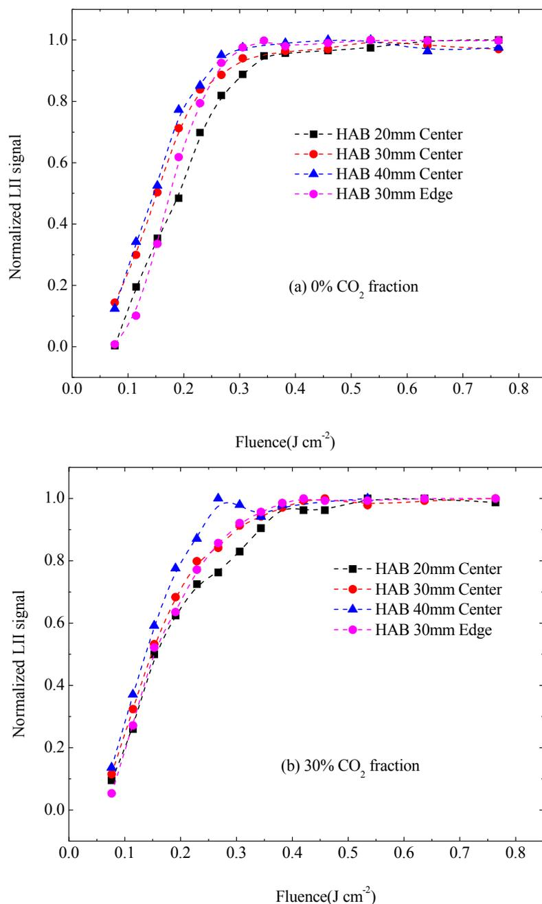
**Fig. 4.** LII fluence curves of flames fueled with gases containing (a) 0%, (b) 30% and (c) 50% volumetric  $\text{CO}_2$  fraction respectively.
