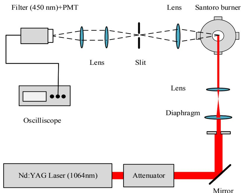
**Fig. 2.** The laser-based measurement platform.
