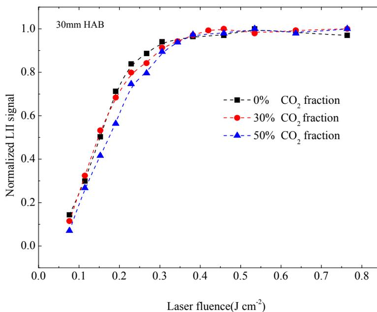
**Fig. 5.** The fluence curves plotted at 30 mm HAB in flames fueled with gases containing different volumetric CO<sub>2</sub> fractions.
