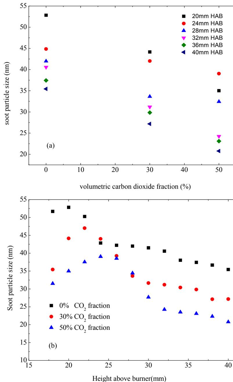
**Fig. 9.** Calculated particle sizes in different flames. (a) The relation between particle sizes and volumetric CO<sub>2</sub> fraction of CO<sub>2</sub>. (b) The relation between particle sizes and the height above the burner.
