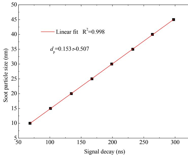
**Fig. 7.** The relation between the soot particle size and the signal decay. Signal decays were calculated through exponential fits to simulated LII decay signals in Fig. 6. A linear function was given to fit this relation.
