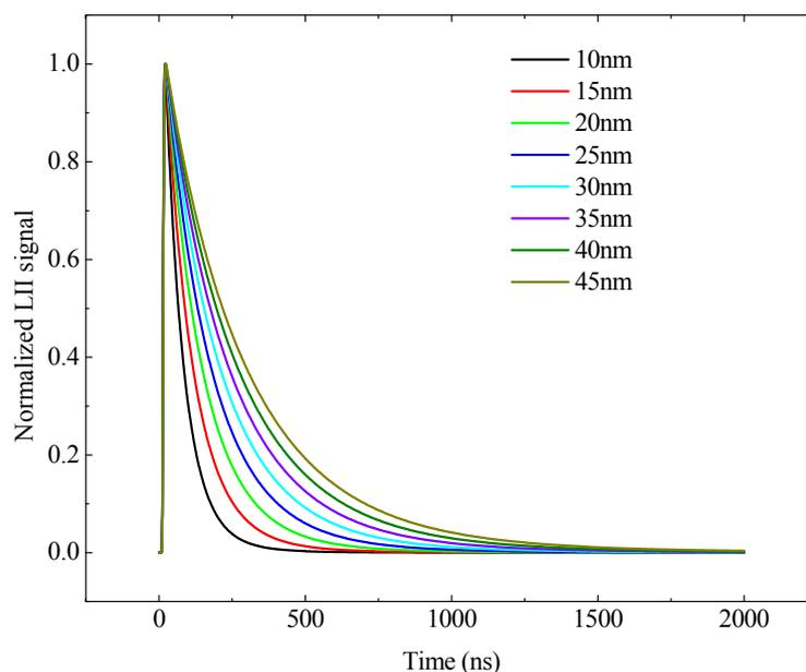
**Fig. 6.** Simulated LII signals of soot particles at different sizes. The input parameters were set as mentioned below.
