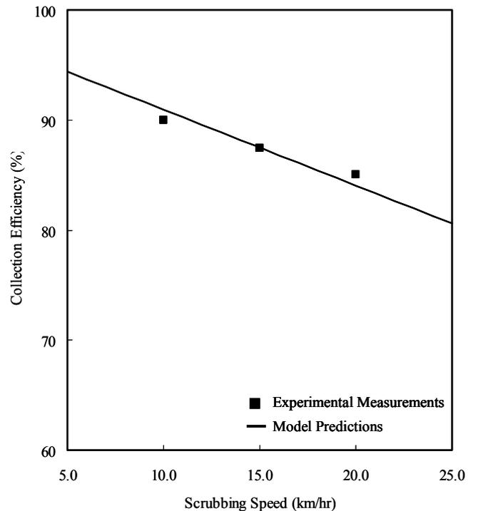
**Figure 11.** Comparison of model-predicted with field-measured collection efficiencies as functions of scrubbing speed.
