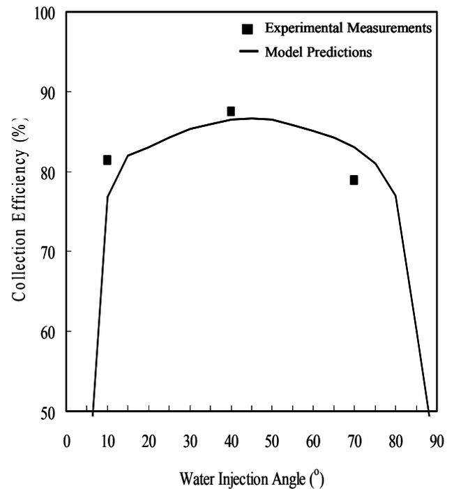
**Figure 15.** Comparison of model-predicted with field-measured collection efficiencies as functions of water injection angle.
