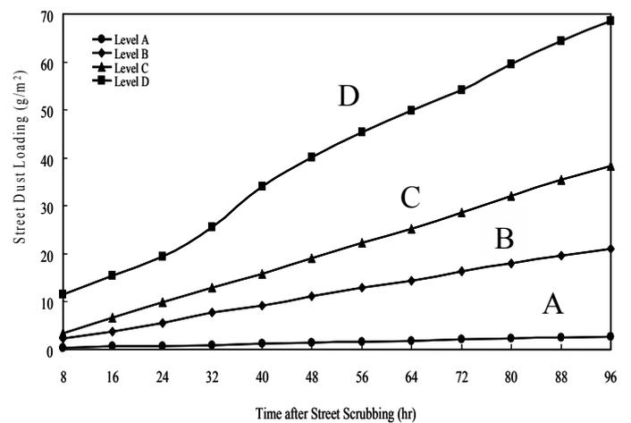
**Figure 1.** Variation of street dust loading with time after street scrubbing.
