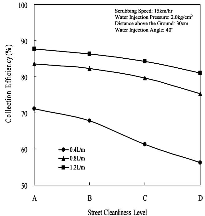
**Figure 4.** Variation of collection efficiency of street dust with water injection loading.
