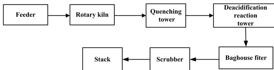
Fig. 2. The system diagram of IHW incineration process.
