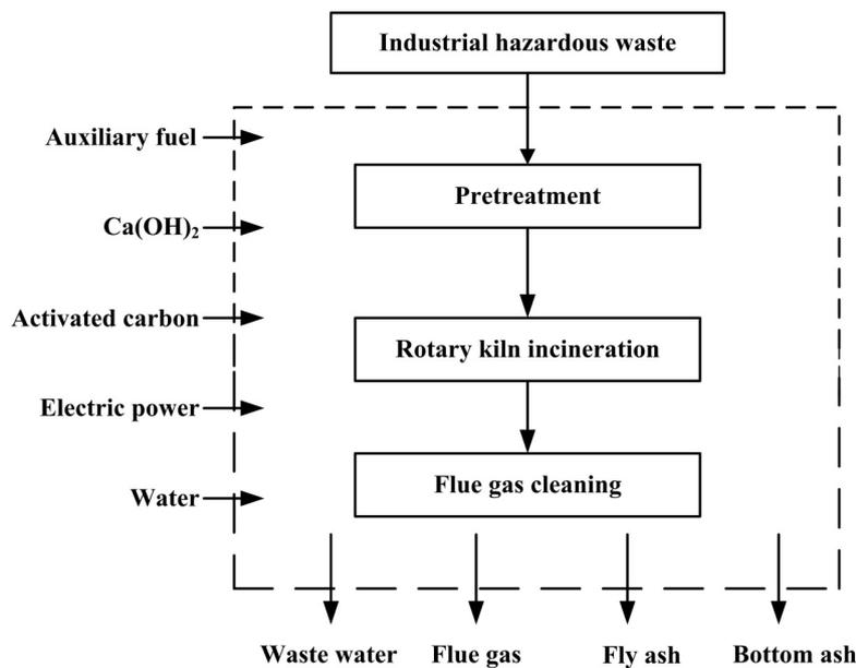
Fig. 1. Model of IHW incineration system.
