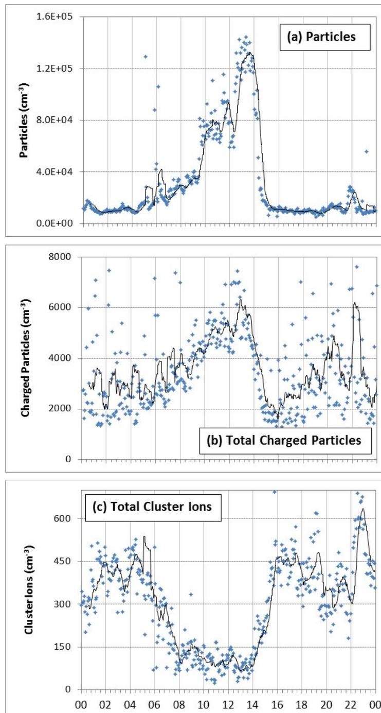
**Fig. 4.** Diurnal variation of particle and ion concentrations on 18 December - a typical bushfire event day. The x-axis shows the time of day in hours. Each point is a 1 min average value and the curves represent 1-hour running averages.
