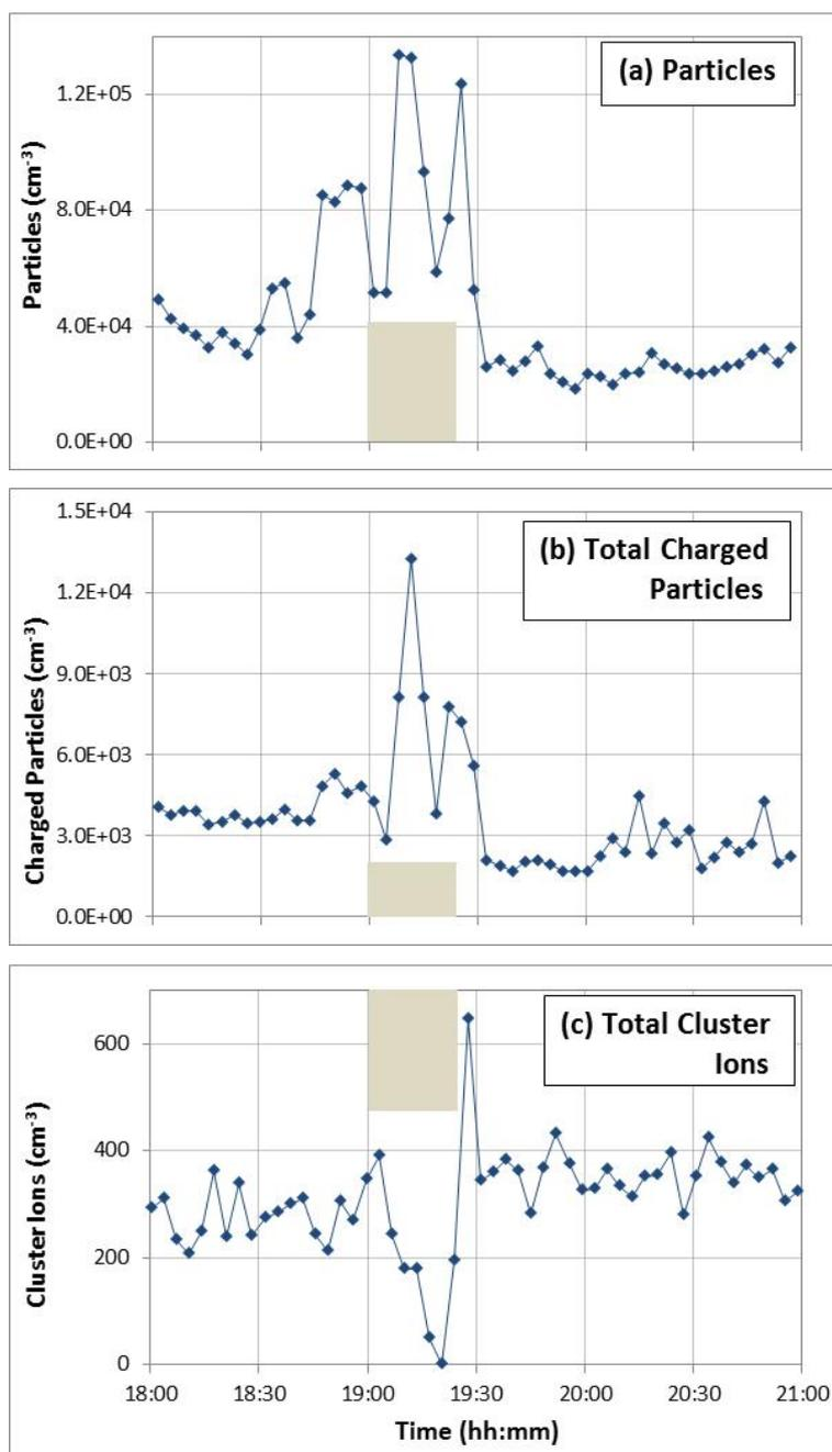
**Fig. 5.** Variation of particle and ion concentrations during the pyrotechnic display on 29 September. The display lasted from 19:00 to 19:25 and this time period is indicated by the shaded area in each graph.
