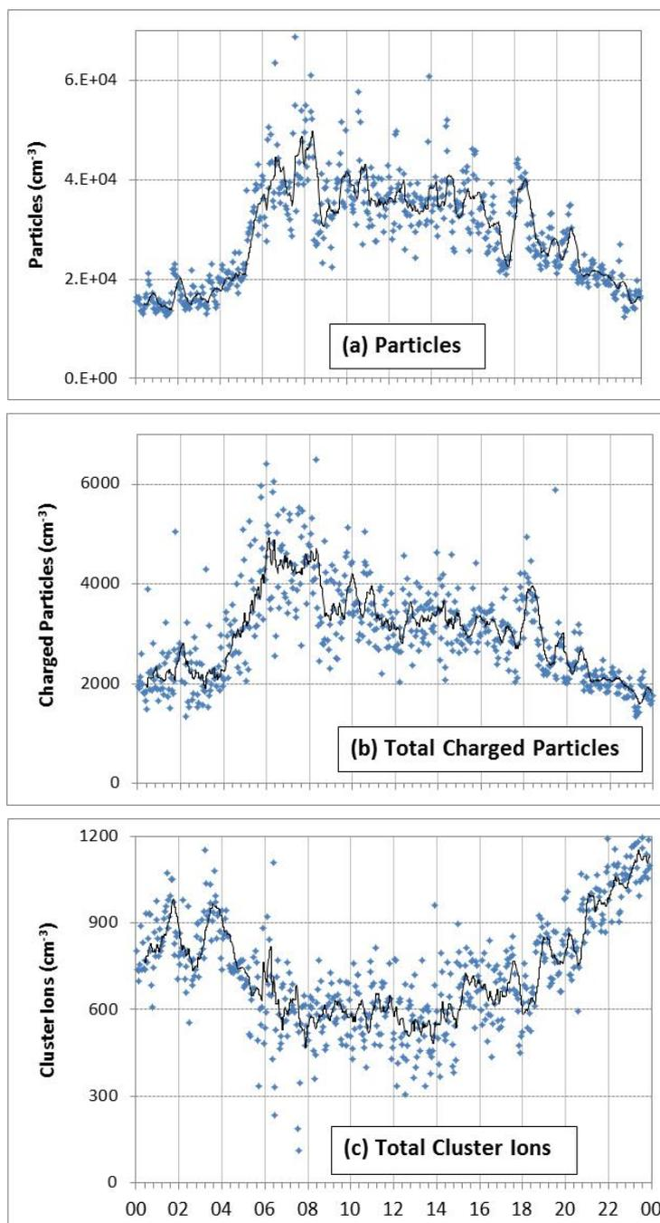
**Fig. 1.** Diurnal variation of particle and ion concentrations on 24 April - a typical day with no particle formation. The x-axis shows the time of day in hours. Each point is a 1 min average value and the curves represent 1-hour running averages.
