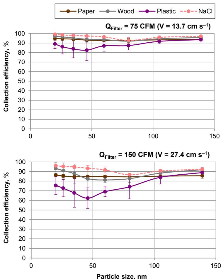
**Fig. 4.** Size-specific collection efficiency of the HVAC filter against combustion and NaCl aerosol particles. Each data point presents an average of 5–6 repeats, error bars present standard deviation.
