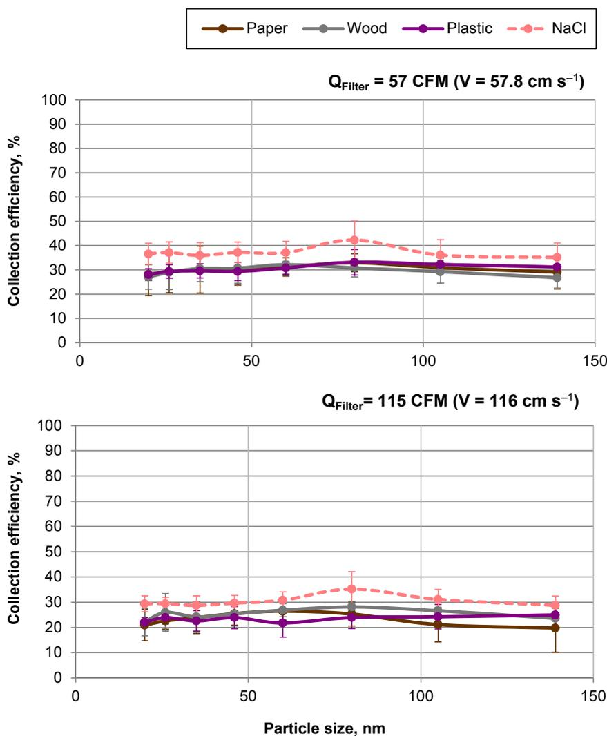
**Fig. 5.** Size-selective collection efficiency of the ACA filter against combustion and NaCl aerosol particles. Each data point presents an average of 5–6 repeats, error bars present standard deviation.
