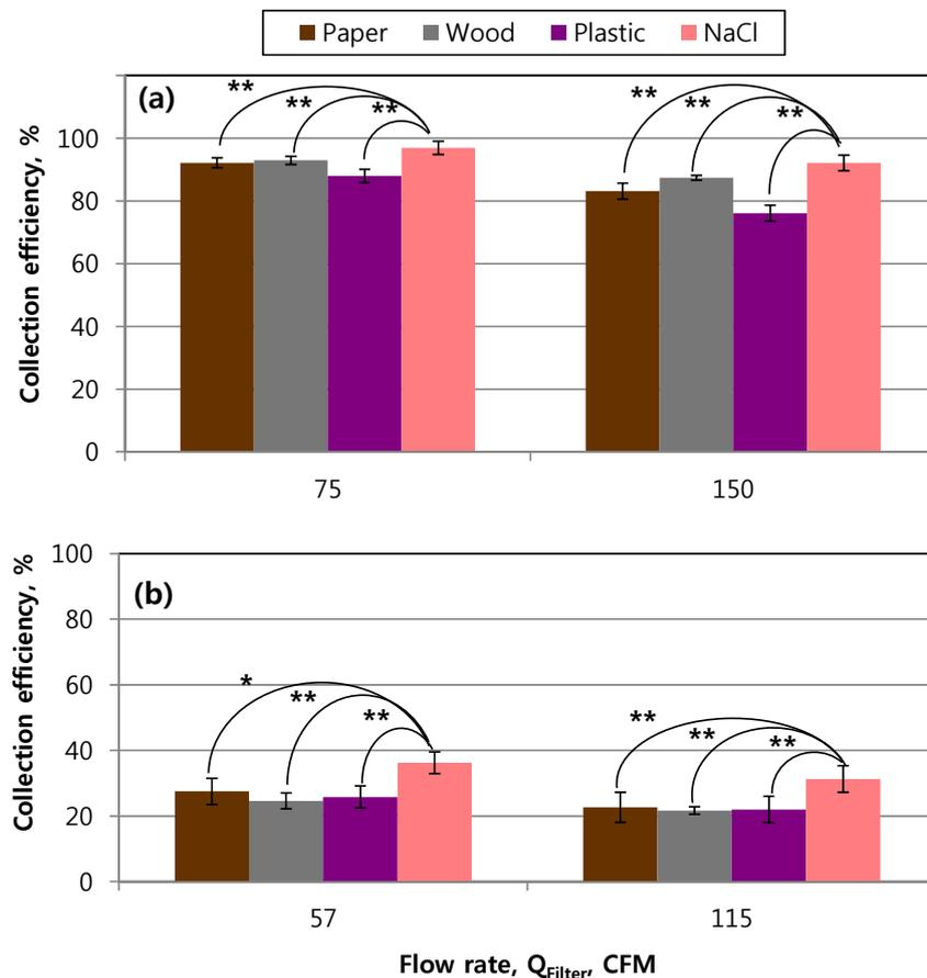
Fig. 3. Total particle collection efficiency of the HVAC (a) and ACA (b) filters determined with a UPC. Symbols \* and \*\* denote statistically significant difference (\*  $p < 0.05$ , \*\*  $p < 0.01$ ). Each data point presents an average of 5-6 repeats, error bars present standard deviation.
