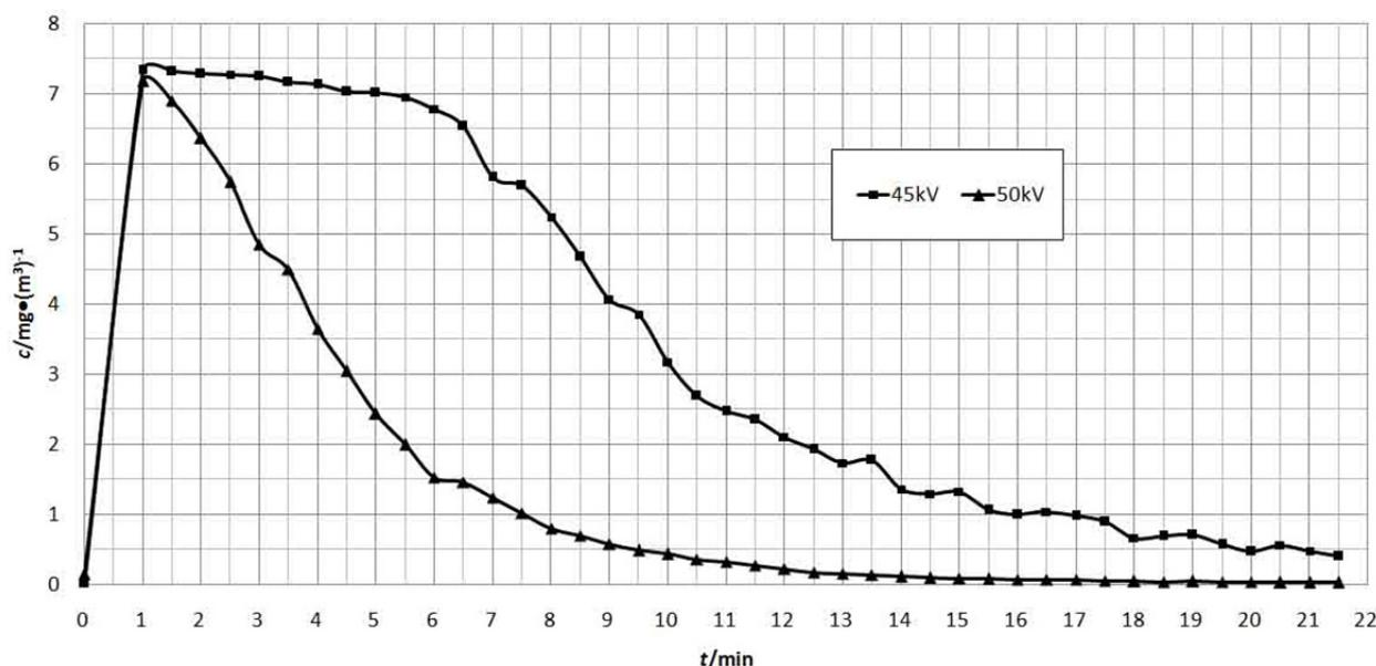
Fig. 5. The value of concentration of  $PM_{2.5}$  with time at different voltages.
