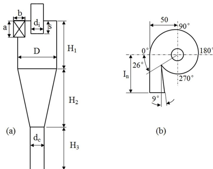
Fig. 1. high-precision Cyclone structure (a) and angular positions (b).
