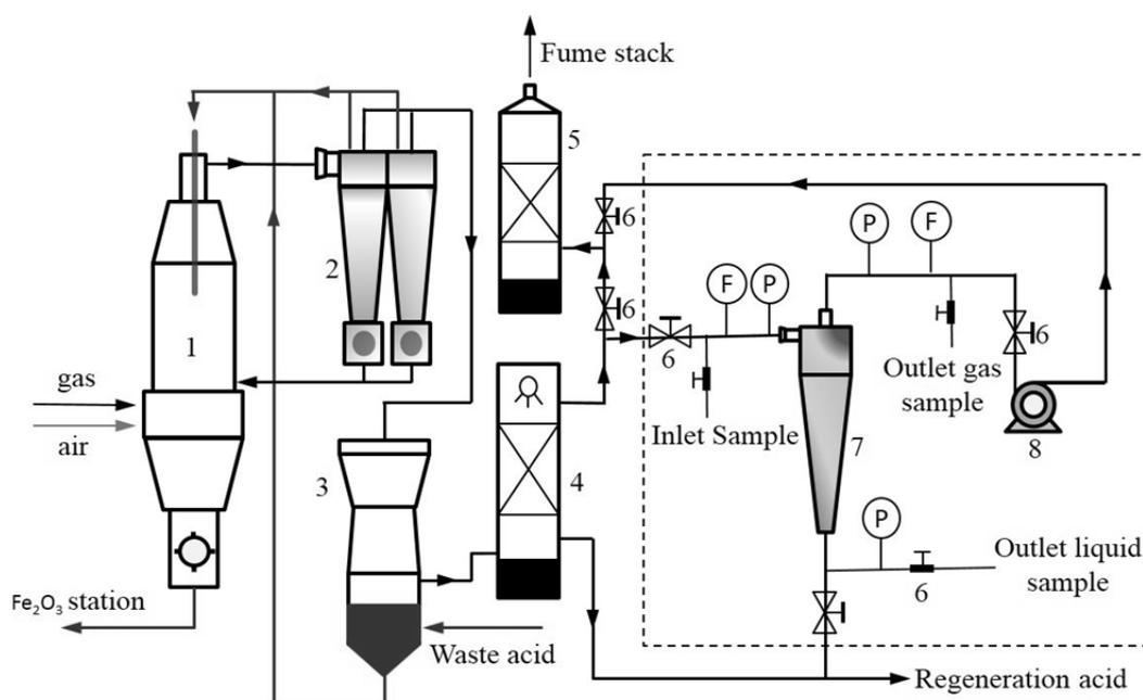
1. Reactor 2. Low precision cyclone separator 3. Preconcentrator 4. Absorption column
