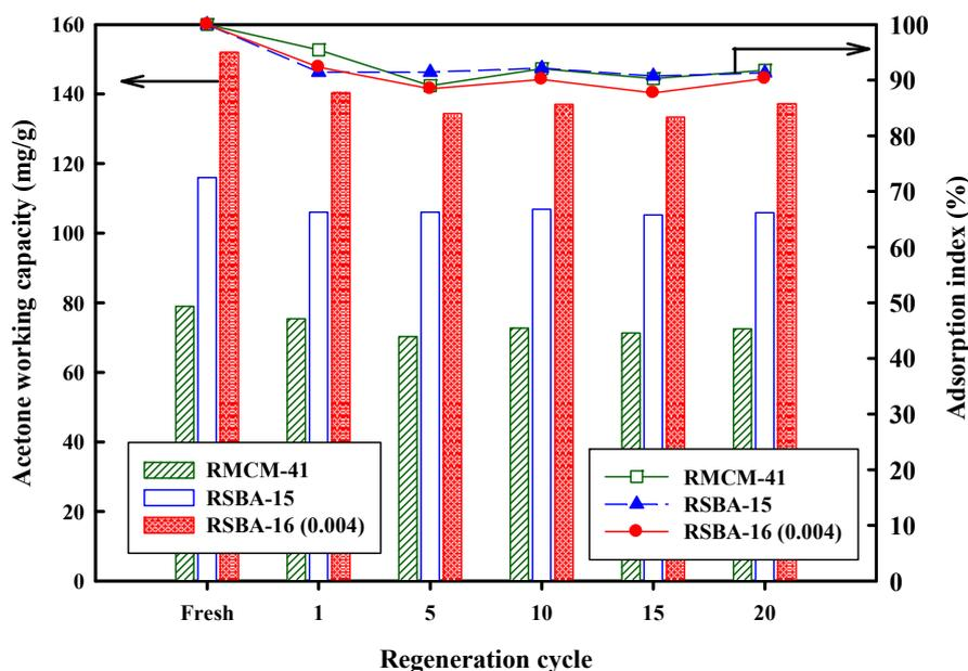
Fig. 8. Cyclic acetone adsorption/desorption performance (working capacity and adsorption index) with RSBA-16(0.004), RMCM-41, and RSBA-15 adsorbents. Cyclic condition: Adsorption temperature: 25°C; Acetone inlet concentration: 1000 ppmv; Desorption temp: 200°C, Desorption time: 30 min.
