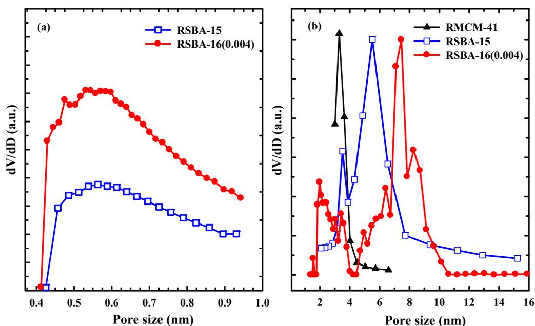
**Fig. 6.** (a) Micropore size distribution of RSBA-15 and RSBA-16(0.004); and (b) Mesopore size distributions for RMCM-41, RSBA-15, and RSBA-16(0.004).
