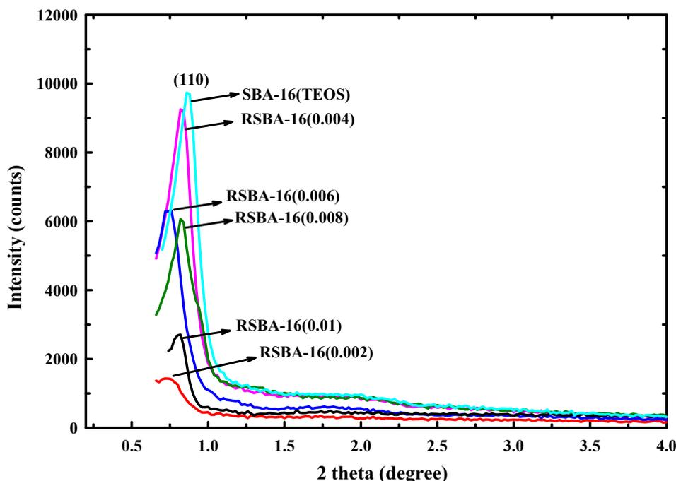
**Fig. 1.** Powder XRD patterns of RSBA-16 prepared at different Surf/Si molar ratios.
