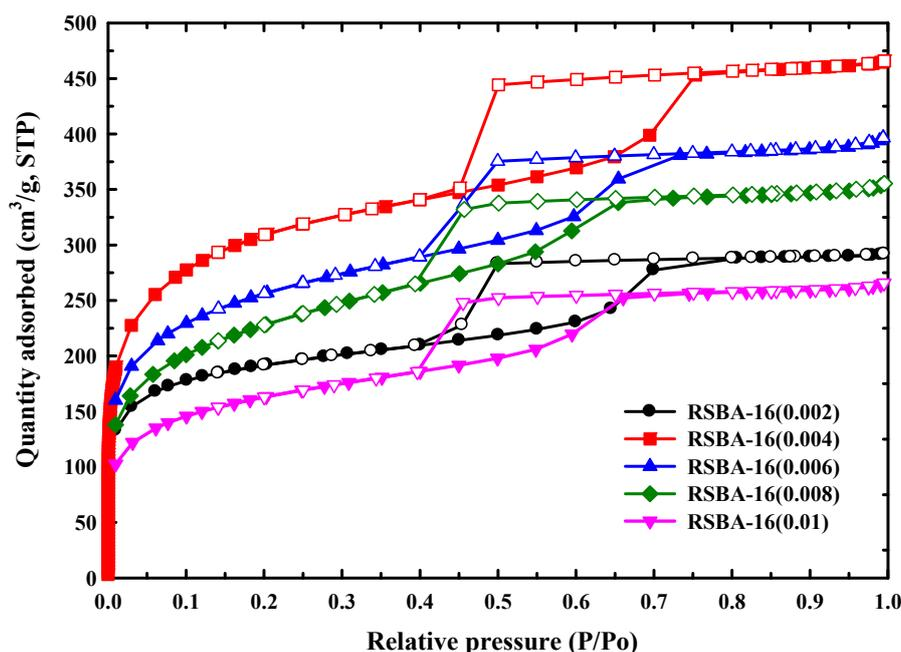
Fig. 2. Nitrogen adsorption-desorption isotherms of RSBA-16 prepared at different Surf/Si molar ratios.
