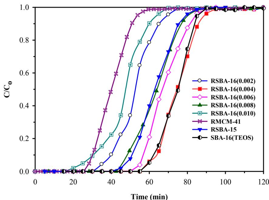
Fig. 3. Acetone breakthrough curves of various adsorbents tested with 1000 ppmv acetone at 25°C.
