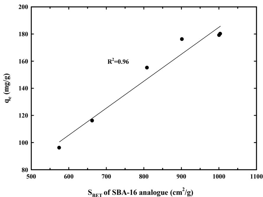
**Fig. 5.** Correlation between the specific surface areas of RSBA-16 adsorbents and their acetone adsorption capacities. Adsorption temperature: 25°C; Acetone inlet concentration: 1000 ppmv.
