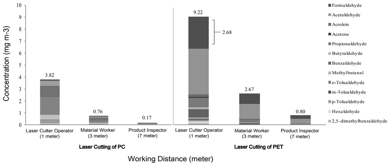
Fig. 7. Total carbonyl concentrations of PC and PET at different exposure distances.
