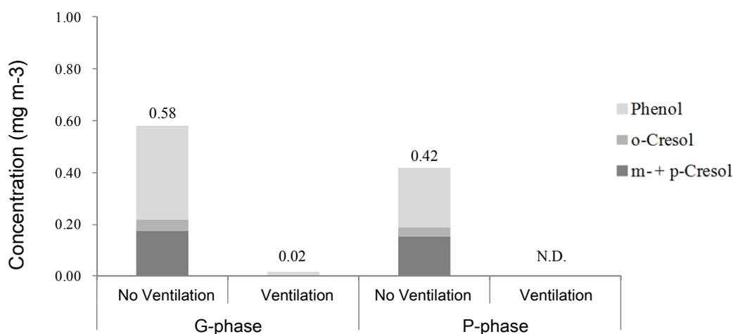
Fig. 13. Total phenol concentrations at different ventilation conditions during laser cutting of PC.
