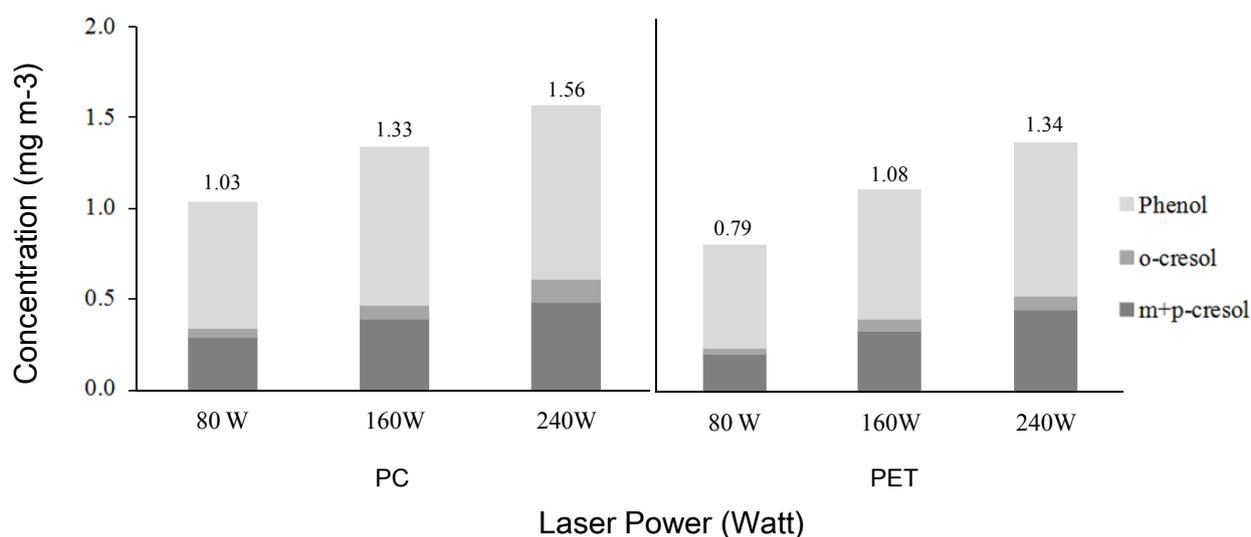
**Fig. 6.** Total phenol concentrations of PC and PET at different laser powers.
