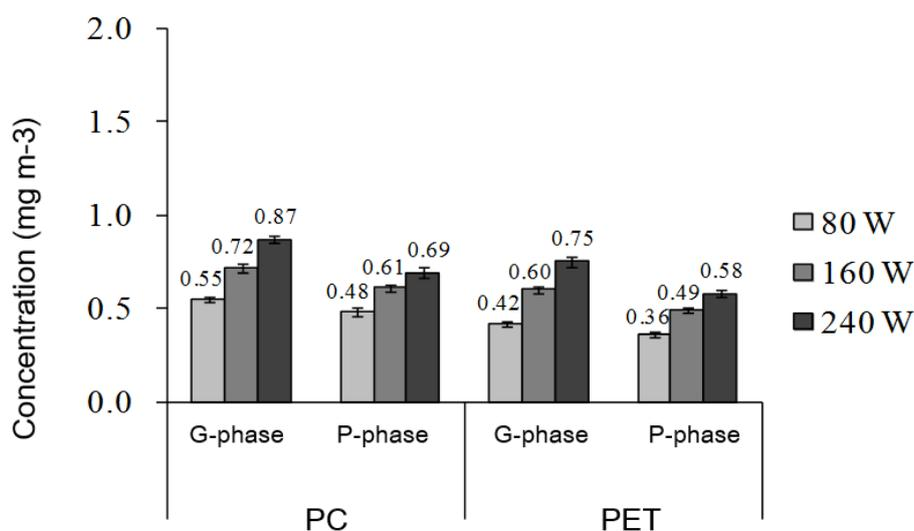
**Fig. 5.** The trends of the gas and particle phases of phenols of PC and PET at different laser powers.
