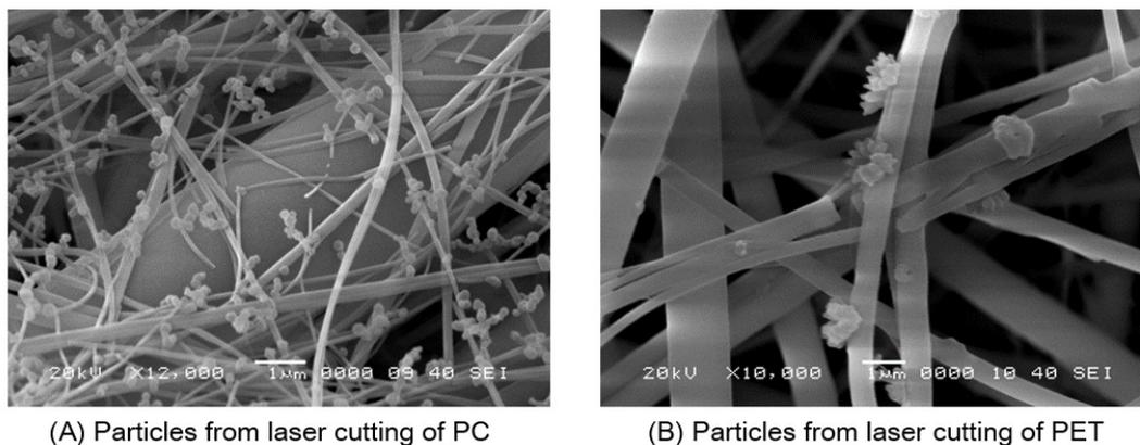
Fig. 1. Particle structure of PC and PET at laser power 240 W.
