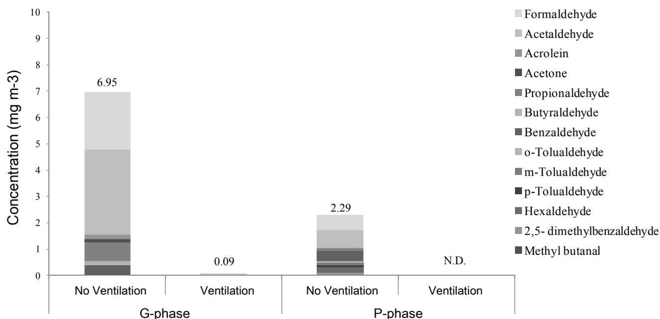
Fig. 12. Total carbonyl concentrations at different ventilation conditions during laser cutting of PET.
