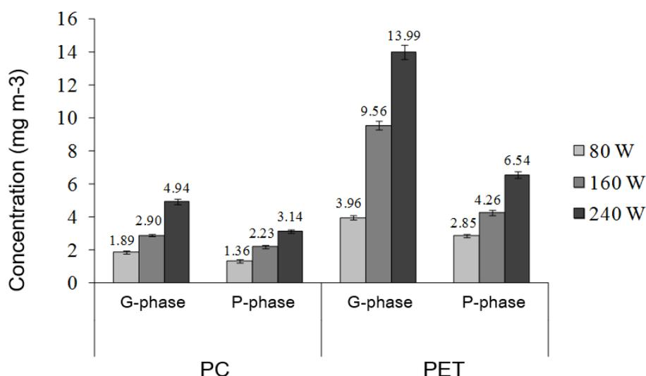
Fig. 3. The trends of the gas and particle phases of carbonyls of PC and PET at different laser powers.
