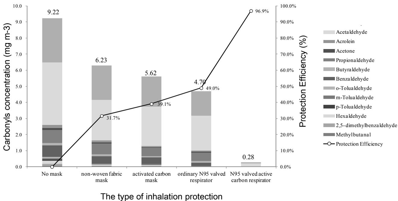
Fig. 10. Total carbonyl concentrations with different masks during laser cutting of PET.
