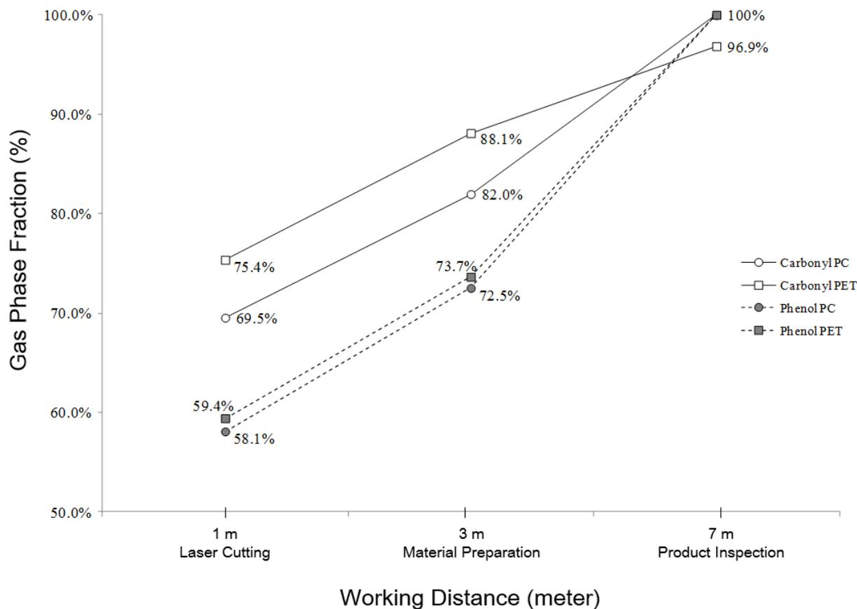
Fig. 9. Total phenol concentrations of PC and PET at different exposure distances.
