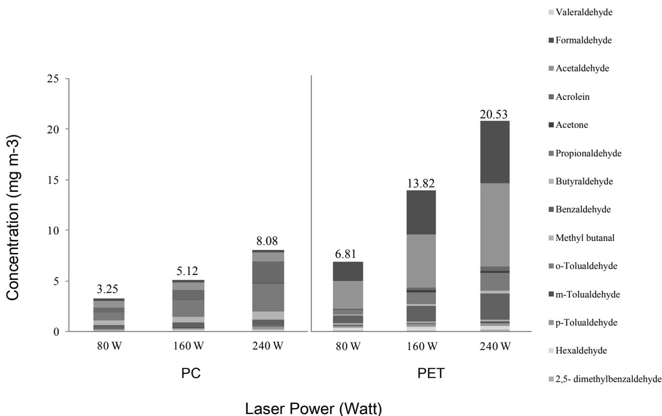
Fig. 4. Total carbonyl concentrations of PC and PET at different laser powers.
