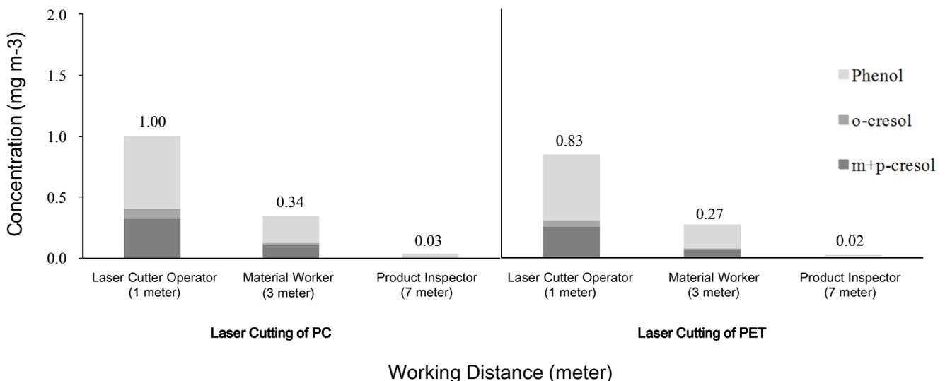
Fig. 8. Total phenol concentrations of PC and PET at different exposure distances.
