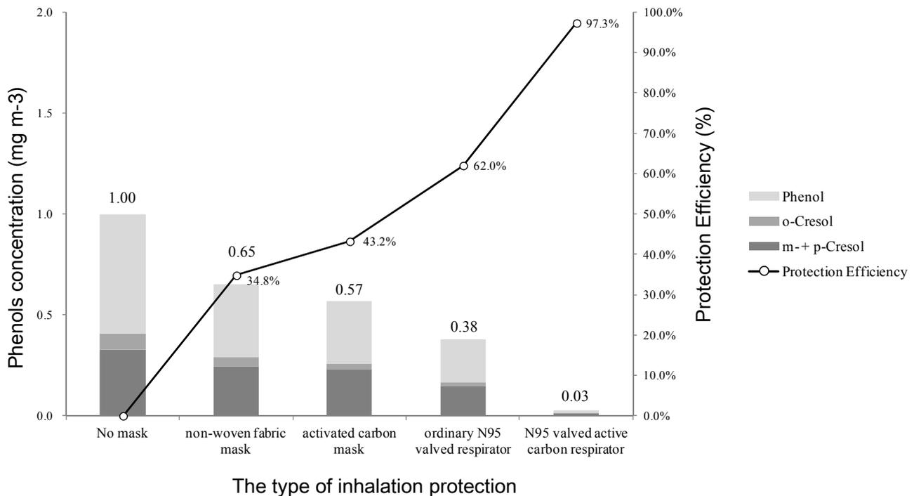
**Fig. 11.** Total phenol concentrations for different masks during laser cutting of PC.
