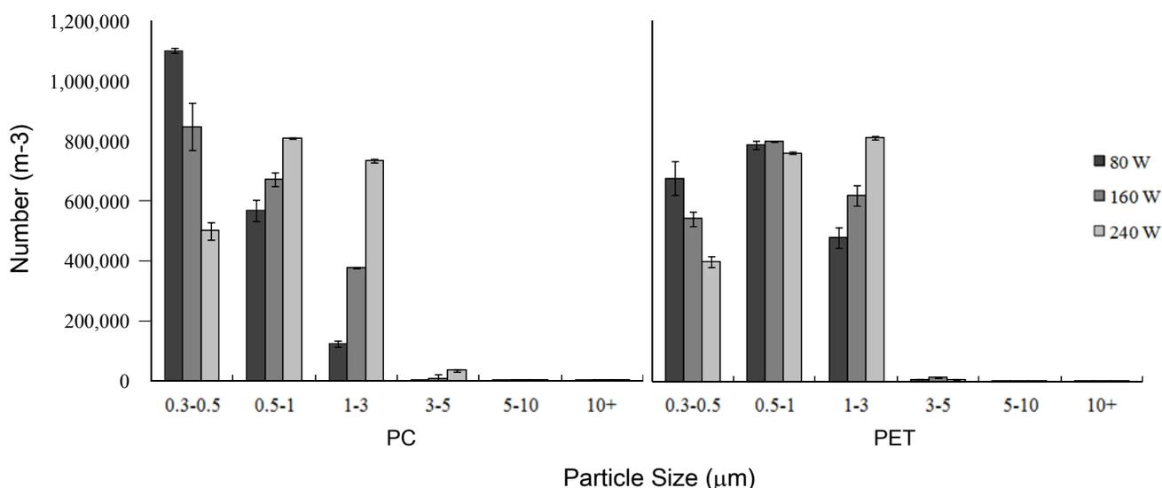
Fig. 2. Particle size distribution of PC and PET at different laser powers.
