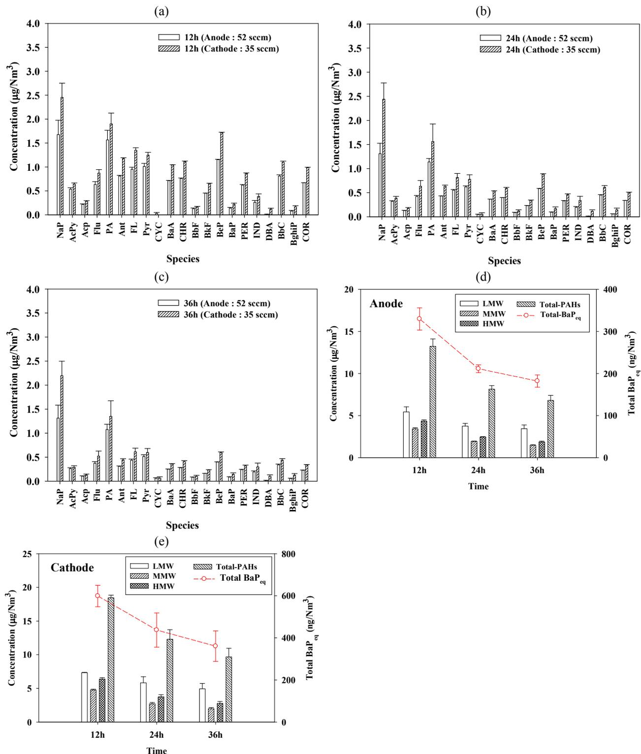
**Fig. 3.** Characteristic profiles of PEMFC emitted PAHs collected at different sampling times (65°C): (a) 12 h, (b) 24 h, and (c) 36 h; concentrations of corresponding LMW-, MMW-, HMW-, and Total-PAHs and Total-BaP<sub>eq</sub> at (d) anode and (e) cathode (n = 3) (E-TEK2).
