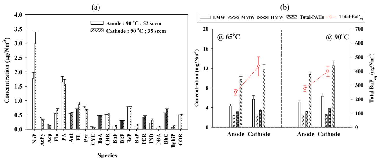
**Fig. 4.** Characteristic profiles of emitted PAHs at 90°C (a) and concentrations of corresponding LMW-, MMW-, HMW-, and Total-PAHs and Total-BaP<sub>eq</sub> at different temperatures (anode =  $52 \text{ mL min}^{-1}$ , cathode =  $35 \text{ mL min}^{-1}$ ) ( $n = 3$ ) (b) (E-TEK2).
