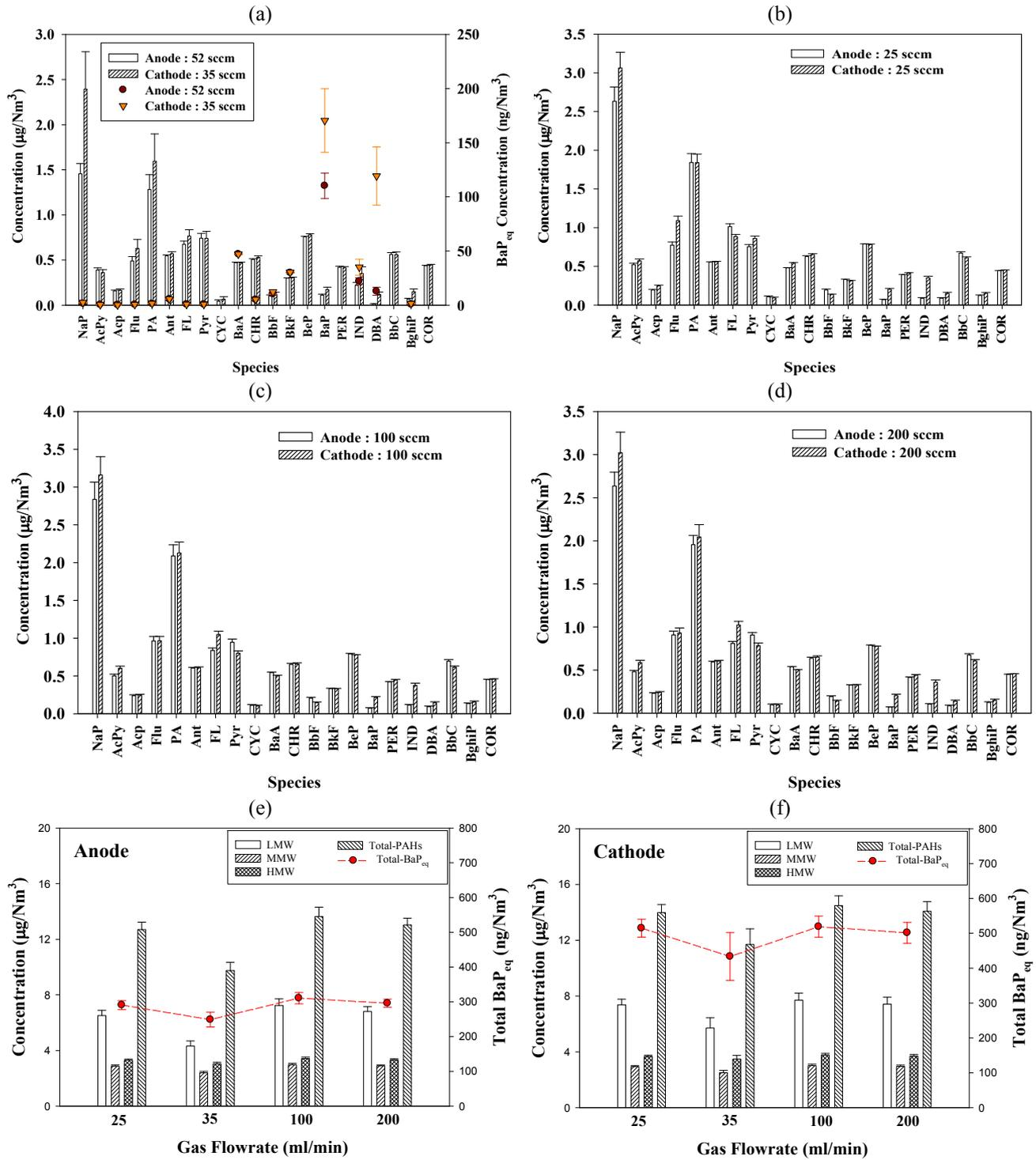
**Fig. 2.** Characteristic profiles of emitted PAHs at different PEMFC flowrates (65°C): (a) anode/cathode = 52/35 mL min<sup>-1</sup>, (b) anode/cathode = 25/25 mL min<sup>-1</sup>, (c) anode/cathode = 100/100 mL min<sup>-1</sup>, (d) anode/cathode = 200/200 mL min<sup>-1</sup>; concentrations of corresponding LMW-, MMW-, HMW-, and Total-PAHs and Total-BaP<sub>eq</sub> at (e) anode and (f) cathode (n = 3) (E-TEK2).
