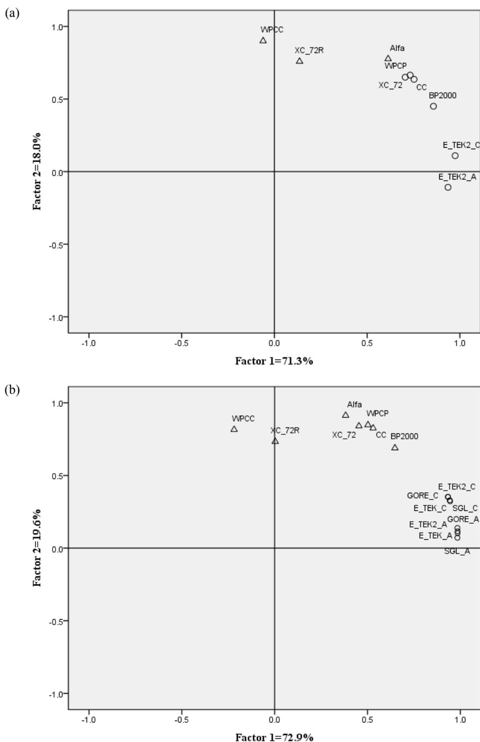
**Fig. 7.** Principle Component Analysis (PCA) for the PAHs of anode/cathode emission gases of PEMFC installed with different MEAs and the PAHs of carbon materials (carbon black: XC-72, XC-72R, Alfa, and BP2000; carbon cloth (CC), water-proof CC (WPCC), and WP carbon paper (WPCP)).
