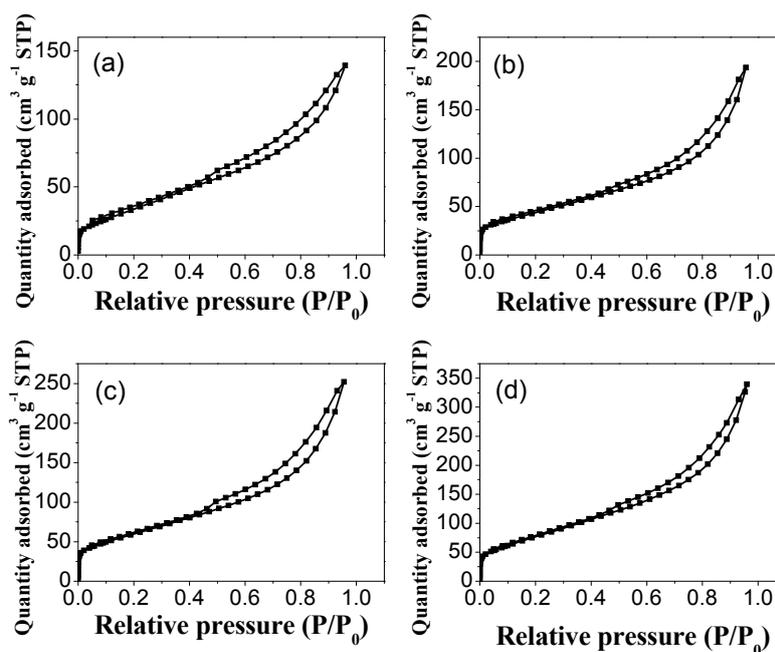
**Fig. 2.**  $N_2$  adsorption-desorption isotherm of G1N0.5 (a), G1N1 (b), G1N2 (c), and G1N3 (d).
