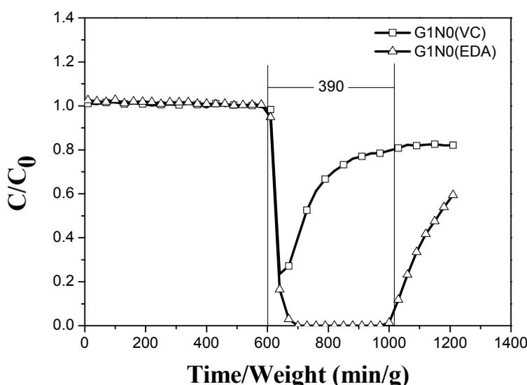
Fig. 6. Breakthrough time of amino-functional aerogels reduced by ascorbic acid and ethylenediamine.
