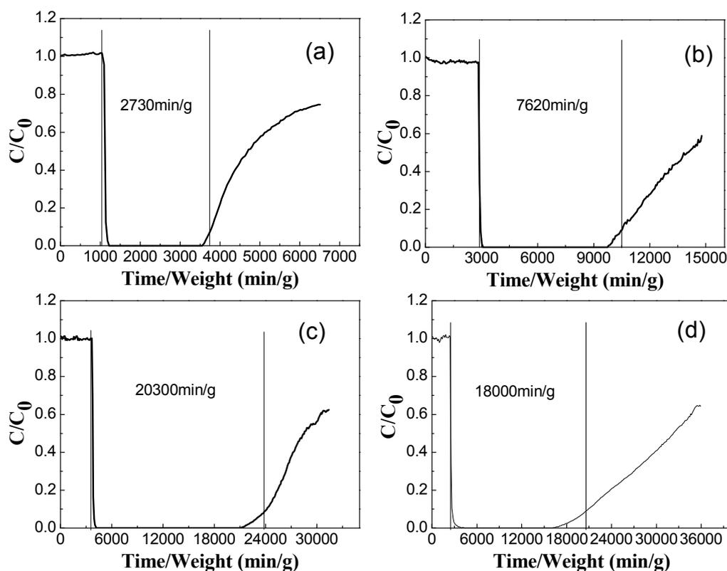
**Fig. 7.** Breakthrough time of amino-functional aerosols with different additions of CNTs. (a) G1N0.5, (b) G1N1, (c) G1N2, (d) G1N3.
