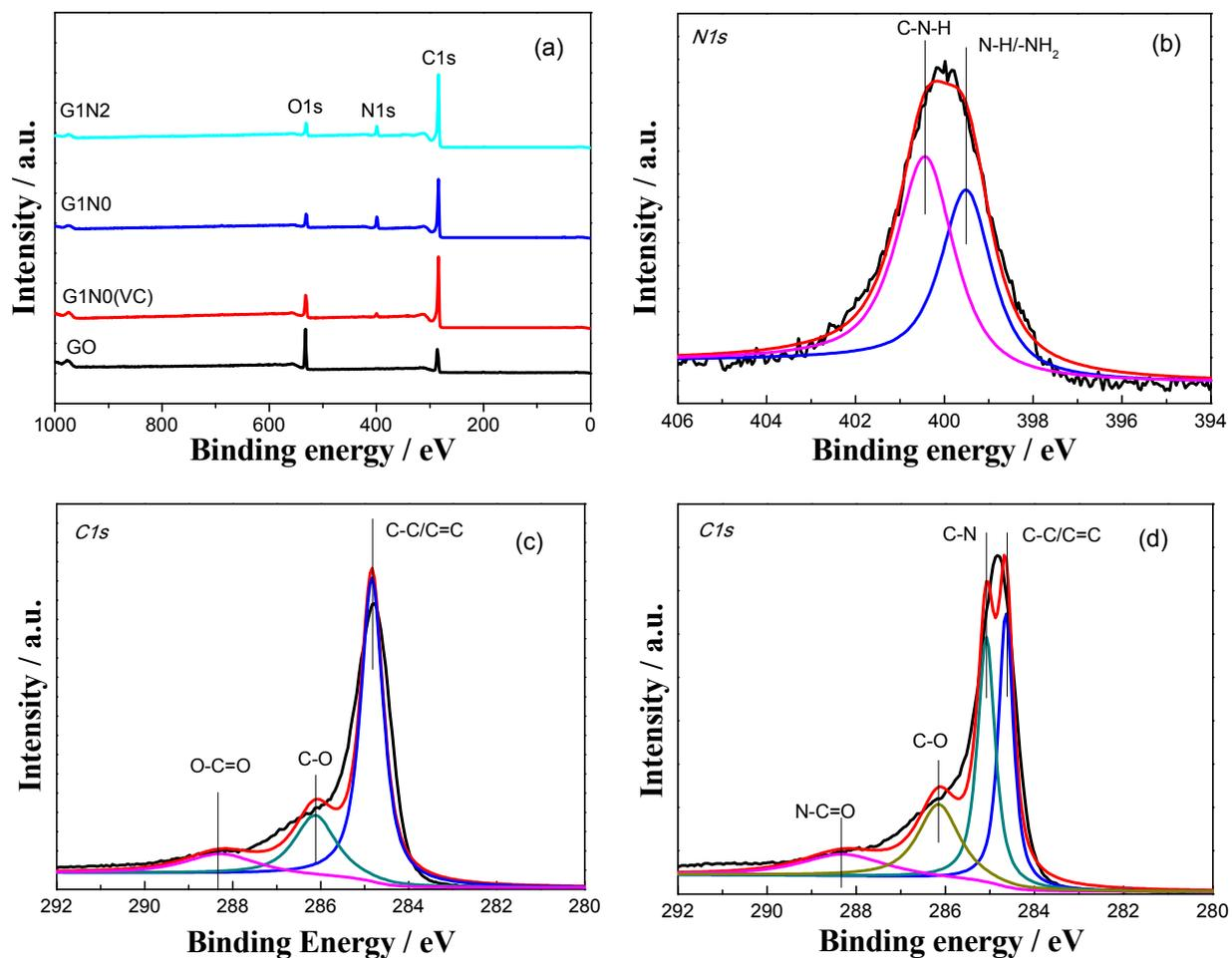
Fig. 5. XPS wide scan (a) of three different aerogels, N1s high-resolution spectra (b) of G1N2, C1s high-resolution spectra (c) of G1N0 (VC), C1s high-resolution spectra (d) of G1N2.
