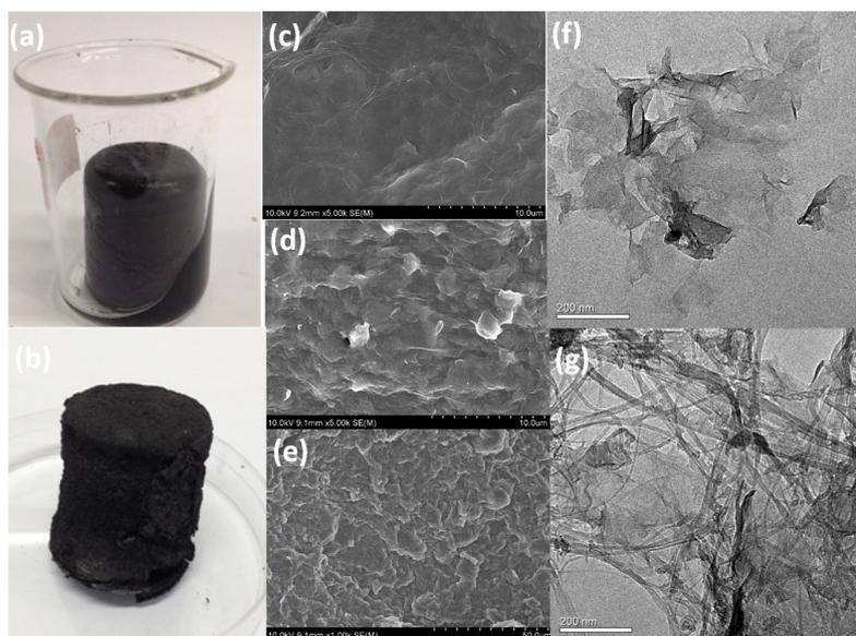
**Fig. 1.** Optical images of amino-functional graphene hydrogel (a) and amino-functional graphene/CNTs aerogel (b); SEM images of G1N0 (VC) (c), G1N0 (d), G1N1 (e), TEM images of G1N0 (f) and G1N1 (g).
