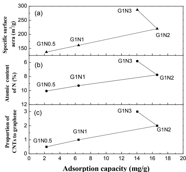
**Fig. 8.** Variation trends of adsorption capacity with proportion of CNTs, atomic nitrogen content and specific surface area.
