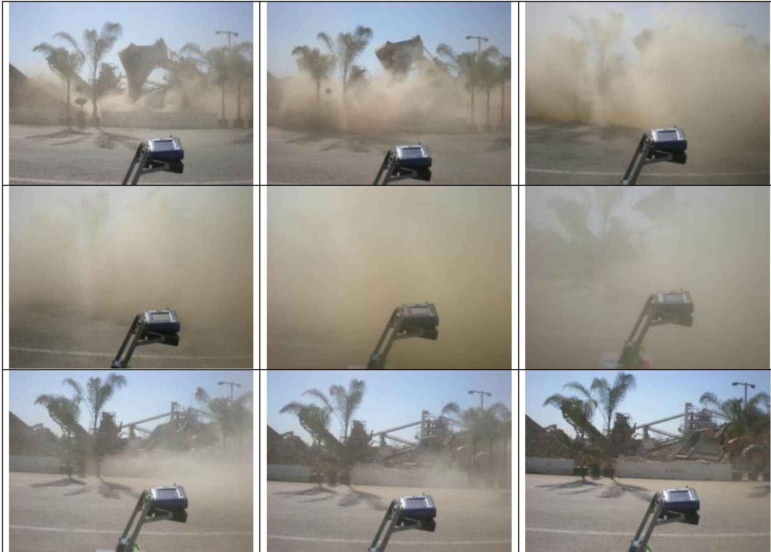
Figure S-5. A simulated fugitive dust event caused by a front-end loader dump near Site A-1 on September 26, 2008. Photographs are ~10 s apart. A slight change in wind direction causes the plume to bypass the sampler with minimal detection as shown in the bottom three panels.
