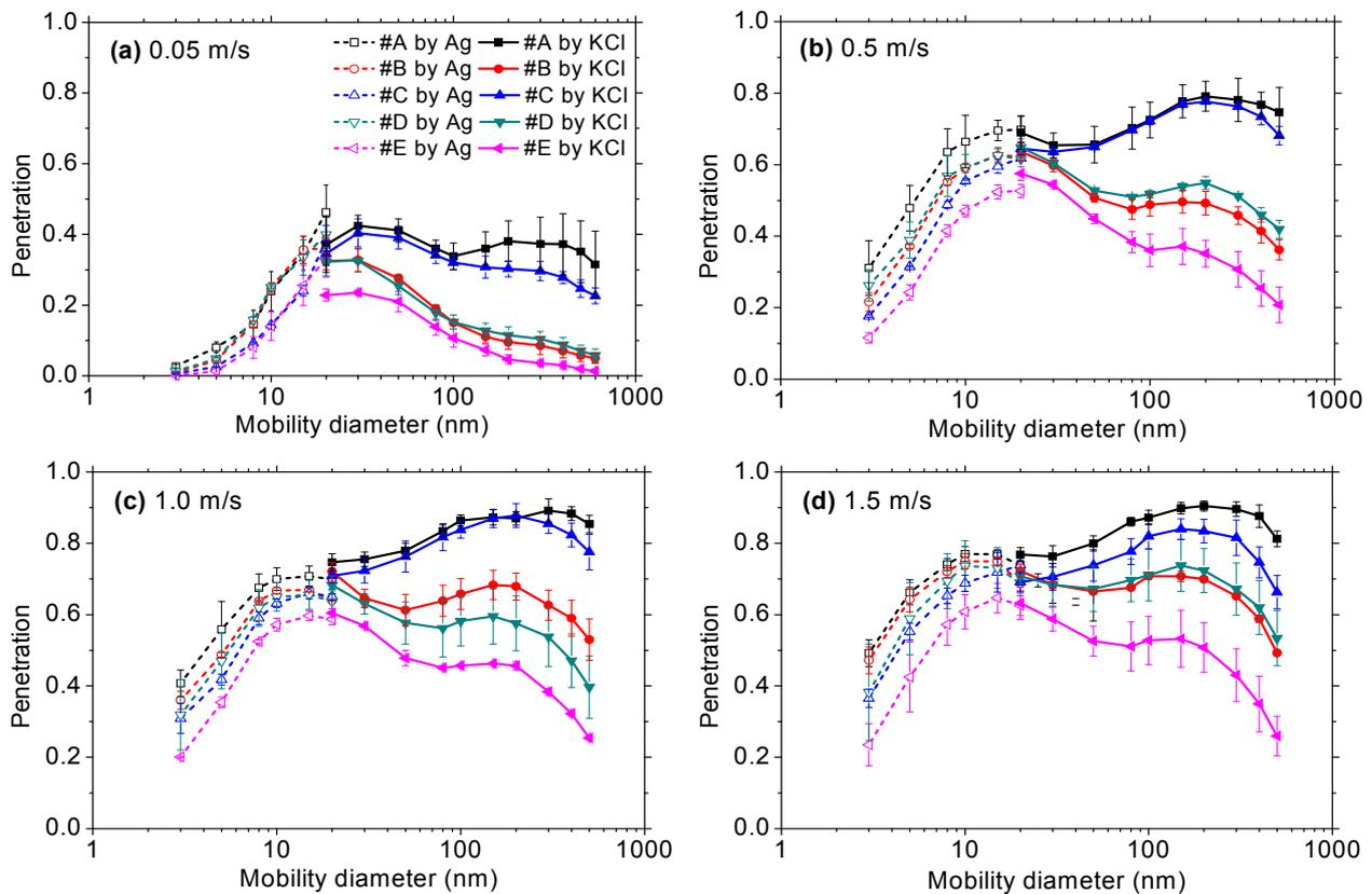
**Fig. 2.** Particle penetration through five electret filter media at face velocities of 0.05 (a), 0.5 (b), 1.0 (c) and 1.5  $\text{m s}^{-1}$  (d).
