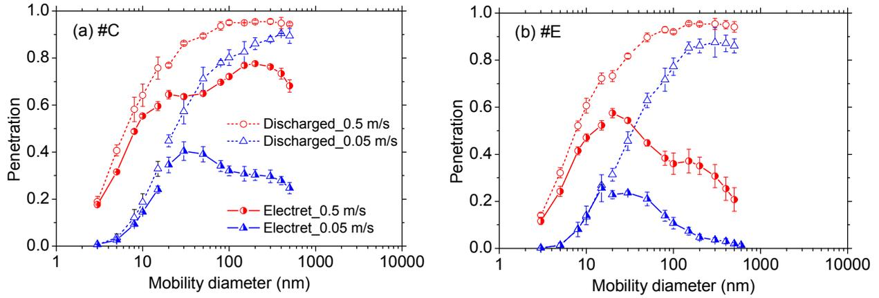
**Fig. 4.** Comparison of penetrations of particle through electret and discharged media #C (a) and #E (b).
