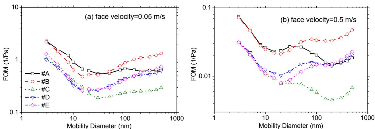
**Fig. 3.** FOM of five electret filter media at face velocities of 0.05 (a) and 0.5 (b).
