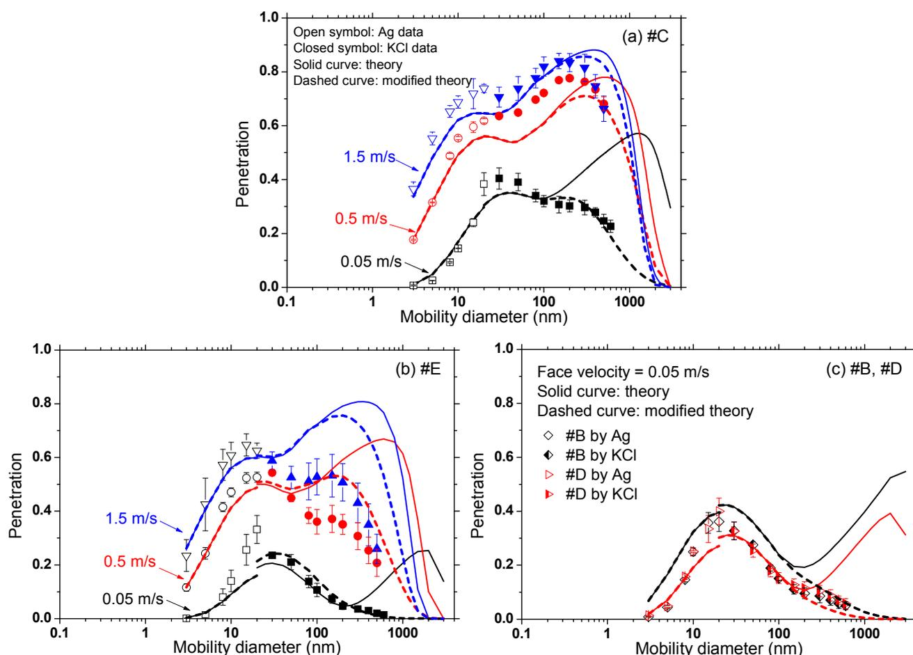
**Fig. 5.** Comparison of experimental and theoretical penetrations of particle through media #C (a) and #E (b) at 0.05, 0.5 and 1.5  $\text{m s}^{-1}$  and media #B and #D (c) at 0.05  $\text{m s}^{-1}$  face velocity.
