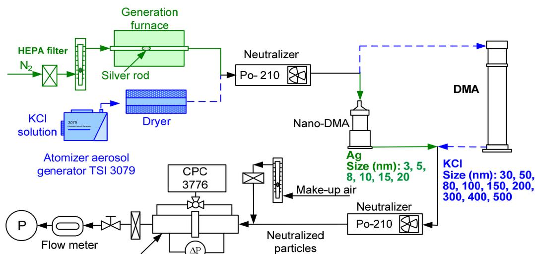
Fig. 1. Experimental setup of particle generation and filtration test.
