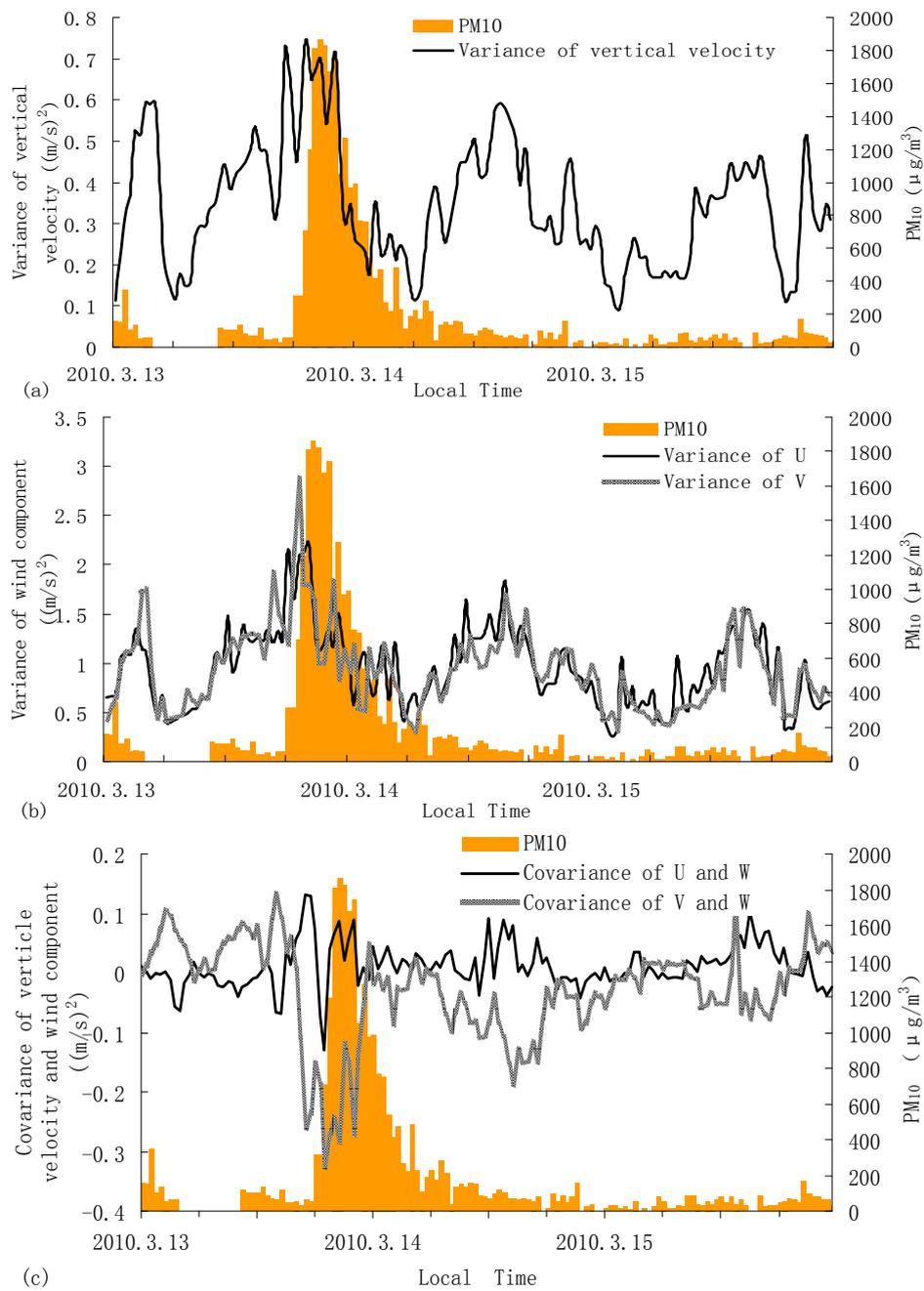
**Fig. 4.** Variation of dynamic factors at the SACOL during 13–15 March 2010: (a) variance of vertical velocity; (b) variance of horizontal wind components; and (c) covariance of vertical velocity and horizontal wind components.
