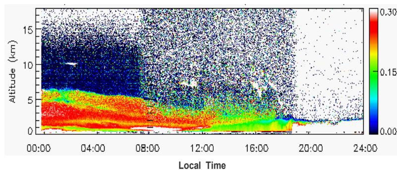
**Fig. 5.** Micro-Pulse Lidar backscatter intensity at the SACOL on 13 March 2010.
