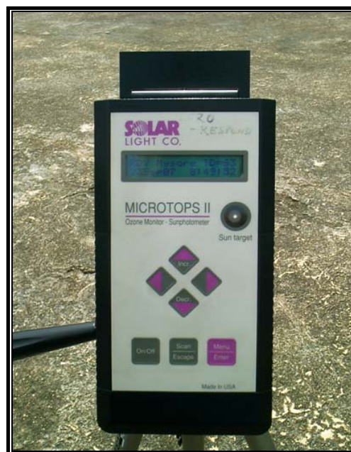
Fig. 1. Tripod mounted MICROTOPS II under action.
