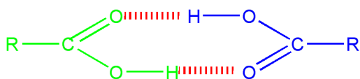
Fig. 4. Carboxyl group at surface of MWCNTs become hydrogen bond. The dotted line stands for hydrogen bond.
